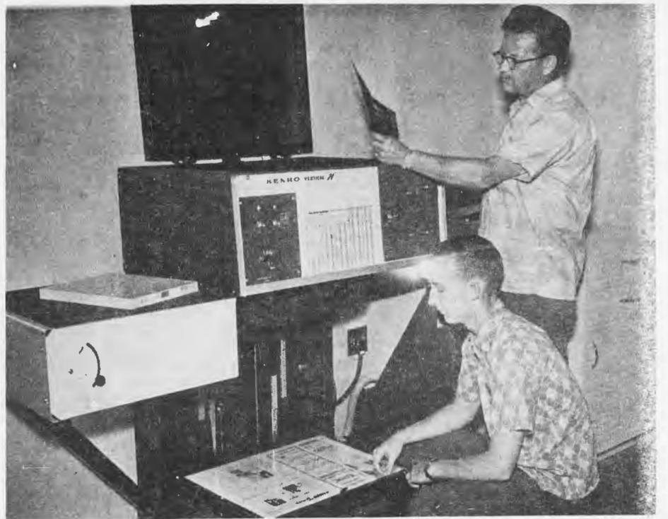
The finished page paste ups are photographed by the fixed-focus camera, resulting in an 18x22 inch negative.
