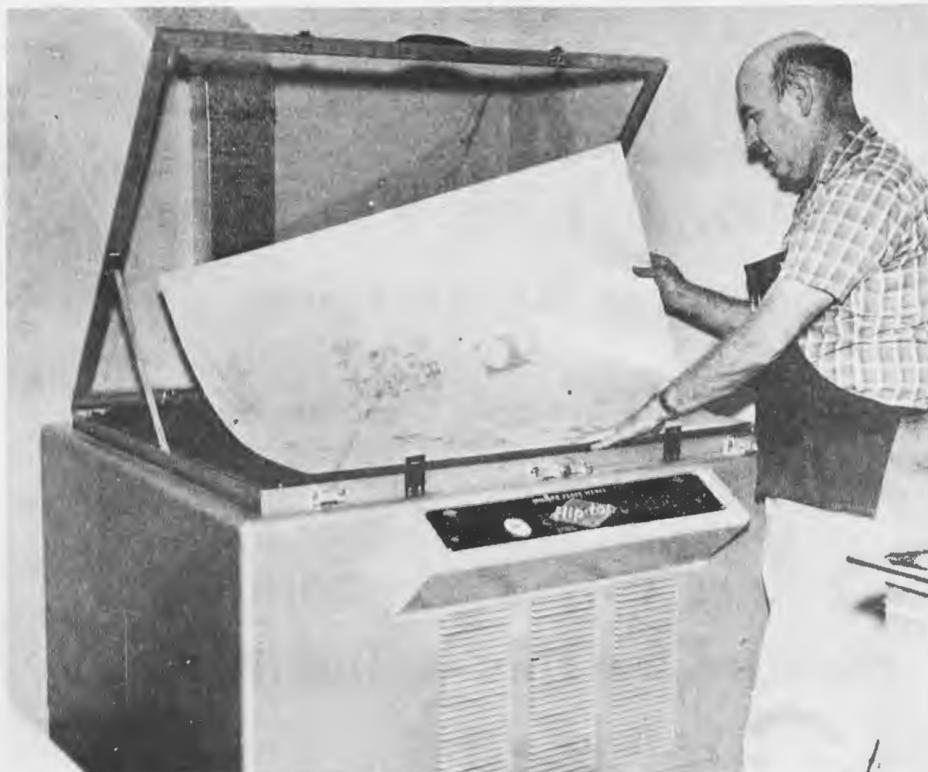
An etched plate is shown being removed from the plate burner. The negative is placed on a pre-treated aluminum plate which is etched by arc light.
