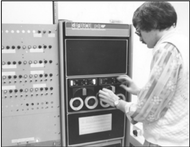
Courtesy EWU Libraries, Archives & Special Collections Business computing in the early 1980s was still dependant on mainframe computers. Data storage was on magnetic tapes and output was on tractor feed paper, both of which are visible in this image.
