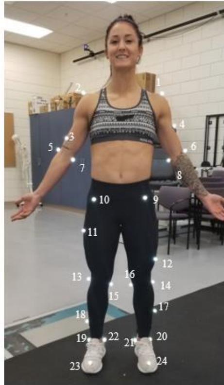
*Figure 9. Placement of reflective markers for the skeletal model. Note markers 25 (L calcaneus) 26 (R calcaneus), and 27 (Sacrum 1) cannot be seen in this image.*
