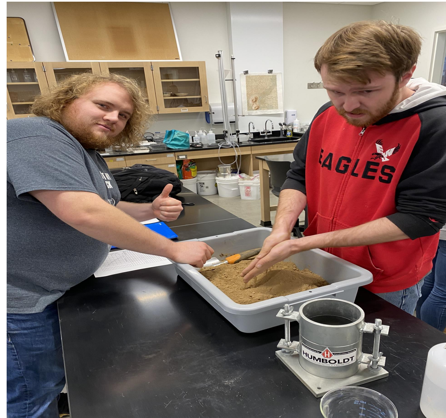
Above is a photo of Spencer and Jarod mixing the soil with water to bring the soil to the maximum water content before standard compaction.
