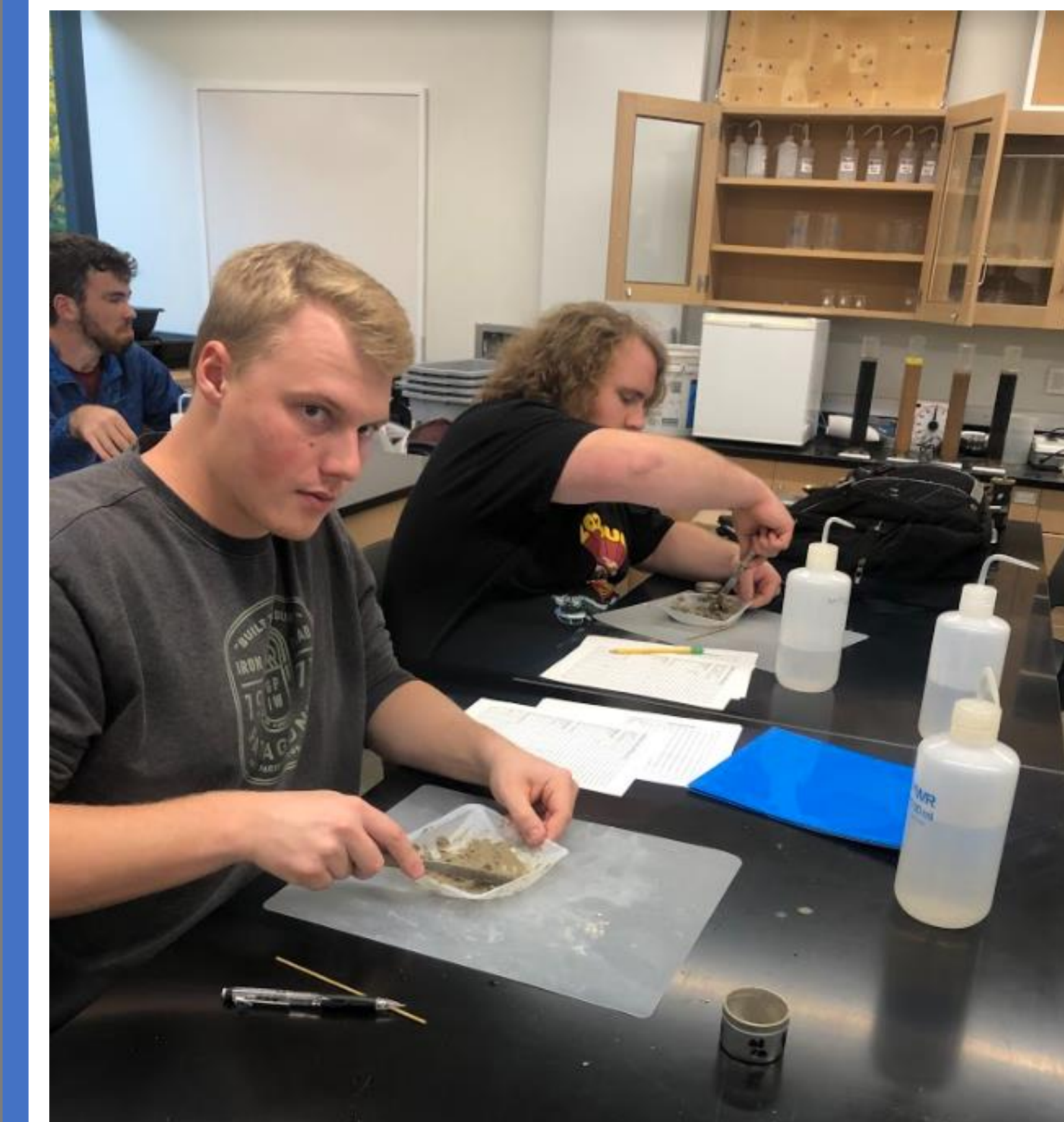
Spencer and Keagan rolling the saturated soil to bring it towards its liquid limit.
