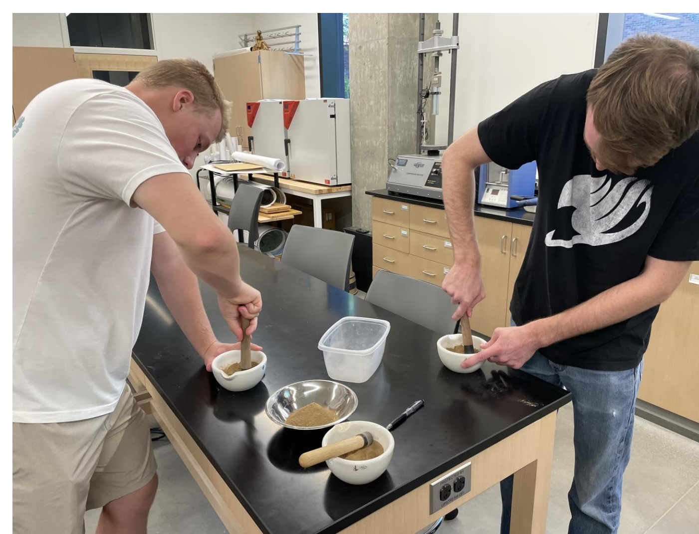
Group members Jarod and Keagan disaggregating soil using pestle and mortar for the sieve analysis.
