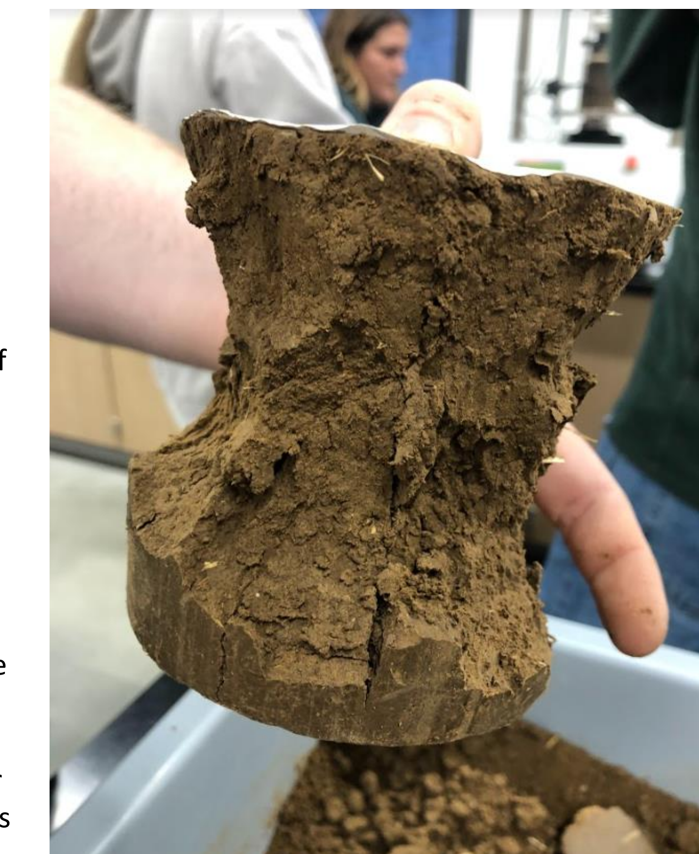
After the unconfined compression test, outer layers of the soil cylinder can be peeled away to show this internal hourglass shape that the soil has taken. This shape shows how the soil reacts against the compressive forces acting on it.
