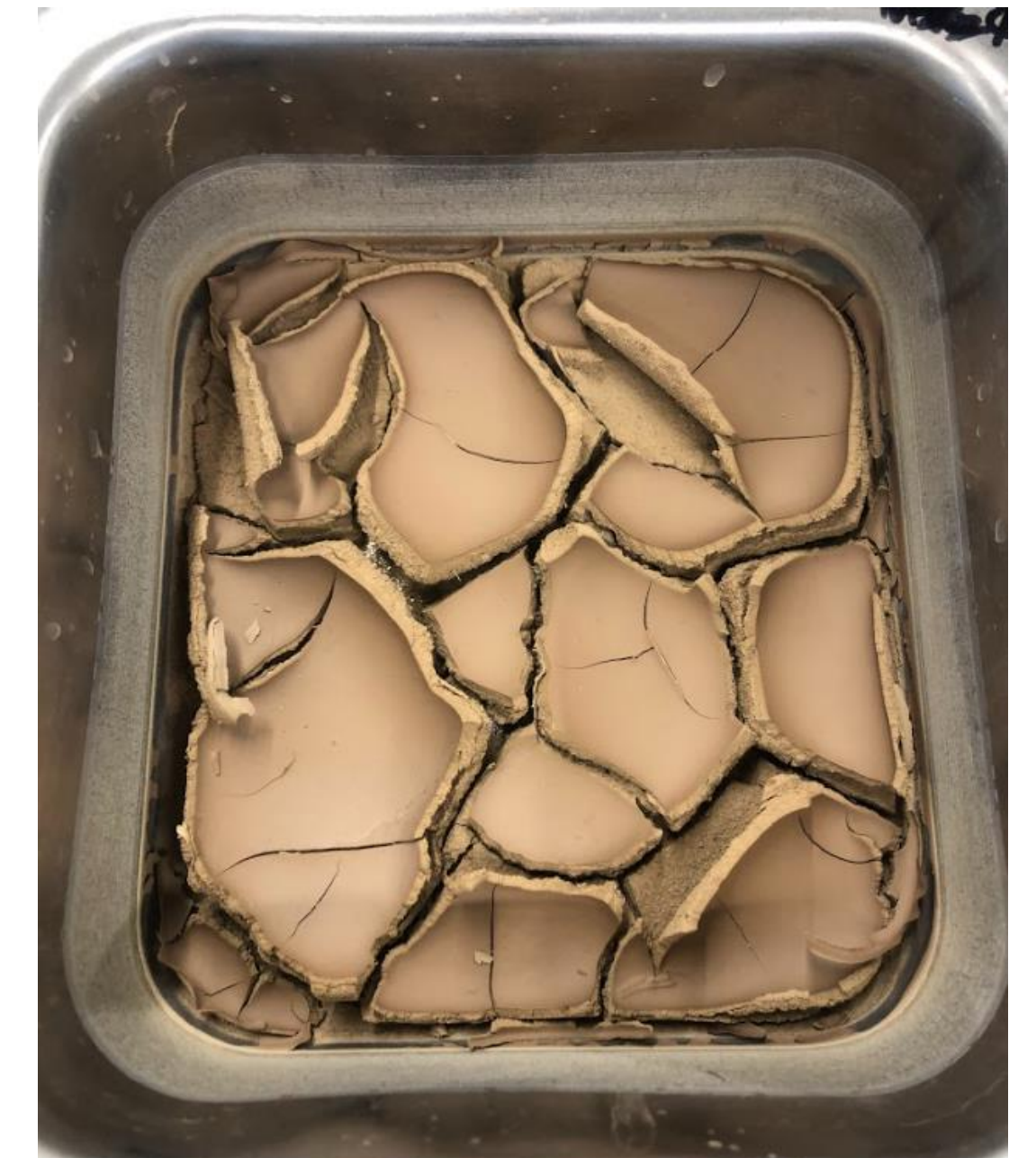
This photo shows what the soil looked like after drying. The mud crack appearance indicates fine clays that are clinging to each other as the soil loses moisture.
