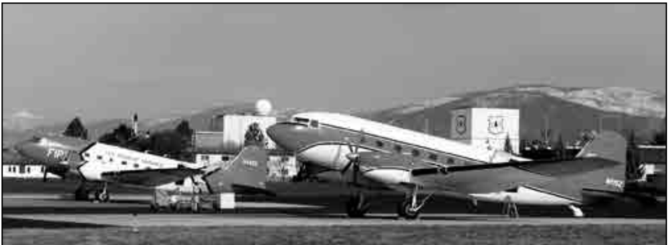
N146Z and N100Z after refitting with turbine engines March 2009. Now numbered N115Z and N142Z. (Courtesy Doug Houston)
