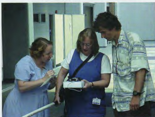
Members of Magnetism Team record data from probe that measures magnetic signature associated with crater feature.
