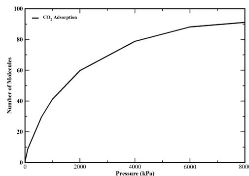
Figure 2: Number of CO<sub>2</sub> molecules adsorbed at various pressures
