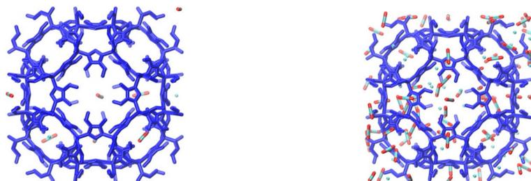
Figure 1: ZIF-93 50/50 mixture of CH<sub>4</sub>/CO<sub>2</sub> at 1 bar (left) and 80 bars (right).
