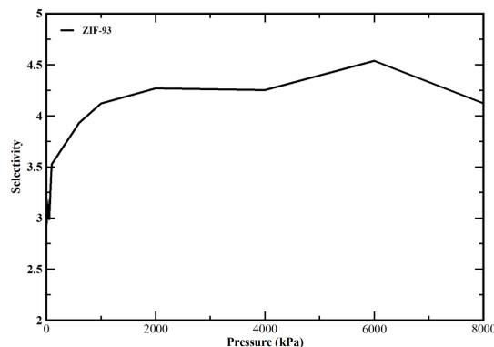
Figure 4: Selectivity of CO<sub>2</sub> over CH<sub>4</sub> for various pressures
