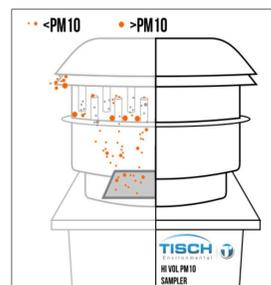
Fig. 2 Photo of high-volume air sampler
