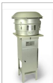
Fig. 1 Photo of high-volume air sampler
