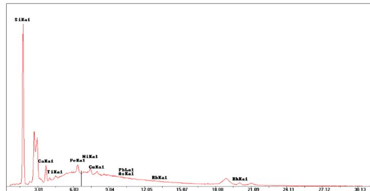
Fig. 5 XRF graph of air filter. Peaks indicate presence of element.
