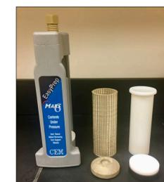
Fig. 8 Digestion vessel assembly
