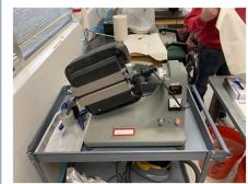
Frantz magnetic separation separation separates remaining magnetic materials (that commonly have similar density to zircon) leaving behind a sample of mostly zircon grains. The Frantz uses a large electromagnet to separate the material into a non-magnetic and magnetic fraction.
