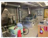
Above: Rock crushing room where we bring in the samples taken from the field then crush them in the chipmunk before running them through the mill which turns the sample into a powder which we then sieve to a specific size for the following steps.
