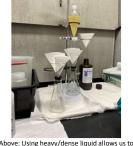
Above: Using heavy/dense liquid allows us to further separate the zircons from other lighter materials that make it through the hydroseperator. The zircons sink to the bottom while lighter materials float.
