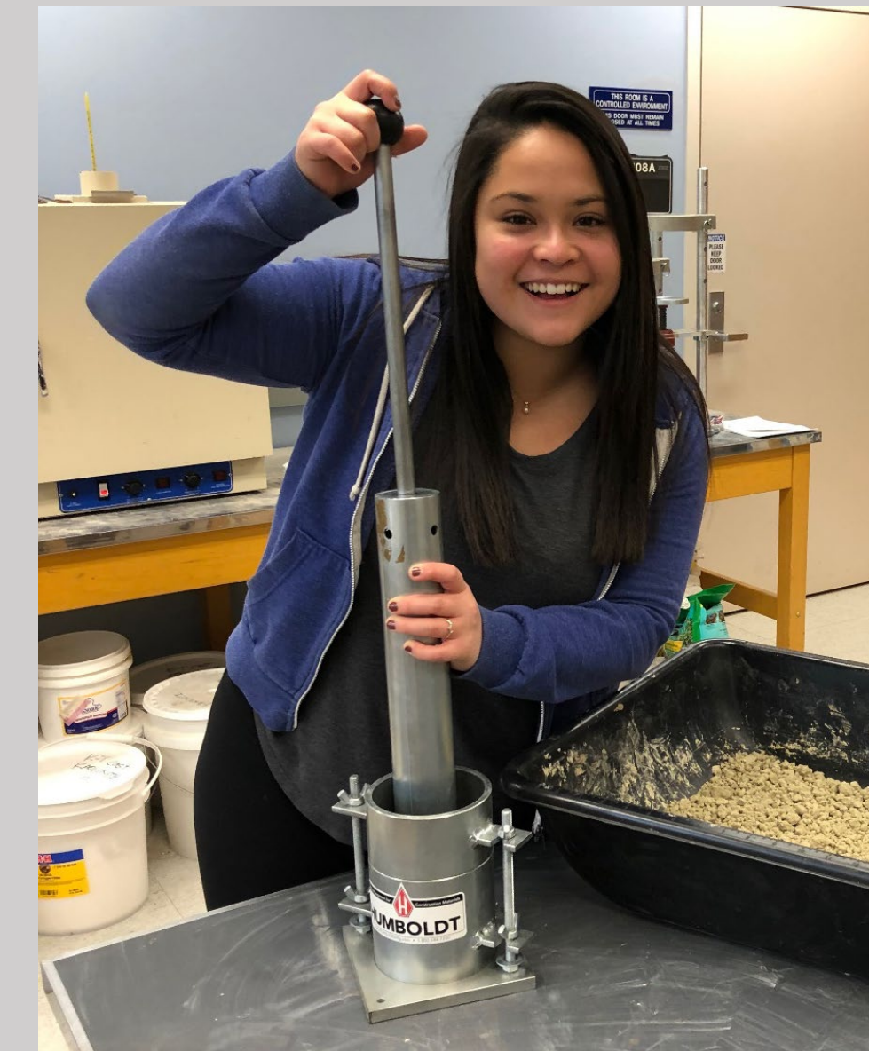
Fig. 3 - Maria holding the 5.5 pound compaction hammer, used to deliver 25 blows per lift. The bin contains the ISC soil.
