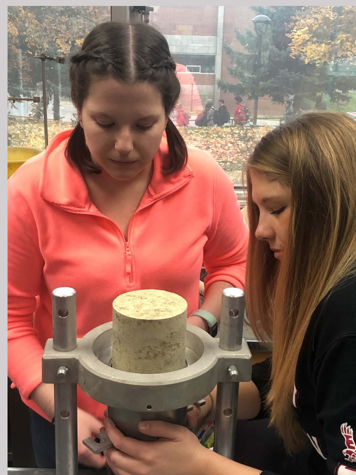
Fig. 4- Rachel and Melissa working together using a hydraulic system to extrude the compacted soil from the cylinder.
