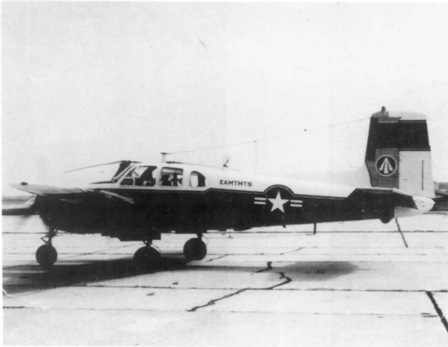
Beechcraft L-23 (a Queen Air). A Command Transport of the type Steve Henault crashed in during Feb. 19, 1971 on Mt. Sanford in Alaska. This type first flew in 1959. It has two Lycoming engines with 320 hp each. Cruising speed is 214 mph at 15,200'; climb rate is 1300 fpm; service ceiling of 27,000'; and a range of 1,445 miles. The U.S. Army ordered substantial quantities of the L-23's in 1960. Photo courtesy of Irene Henault.
