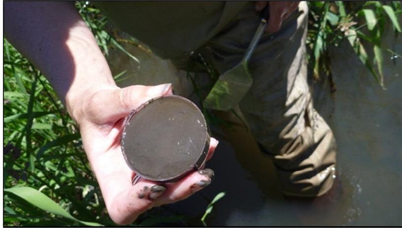
Figure 6. Sediment samples collected in 60 x 15 mm petri dishes.
