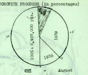
CBI's biggest month, August, registered 394,704 cubic yards of concrete for 27 days of concrete placing. The daily average, however, did not equal the 15,500 yards for each concrete placing day in July.
